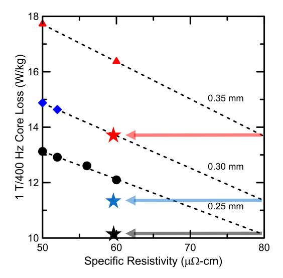
Equivalent core loss at heavier gauges compared to conventional NOES
