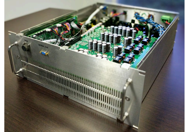
Magnetic Bearing Controller MBC 9600
