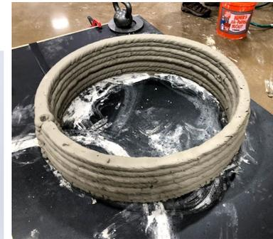
*Concepts and hardware have been developed to evaluate the efficacy of low cost AM for the construction of infrastructure scale structures*
