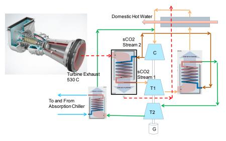
• The turbine currently has an electrical efficiency of 32% at rated power, but with additional steam injection this efficiency can be increased to approximately 37%. Incorporating a sCO2 bottoming cycle will increase total electrical efficiency to around 50%. Special emphasis will be placed on thermo-economic optimization of the cycle, to ensure commercial viability and marketability of the developed system.
