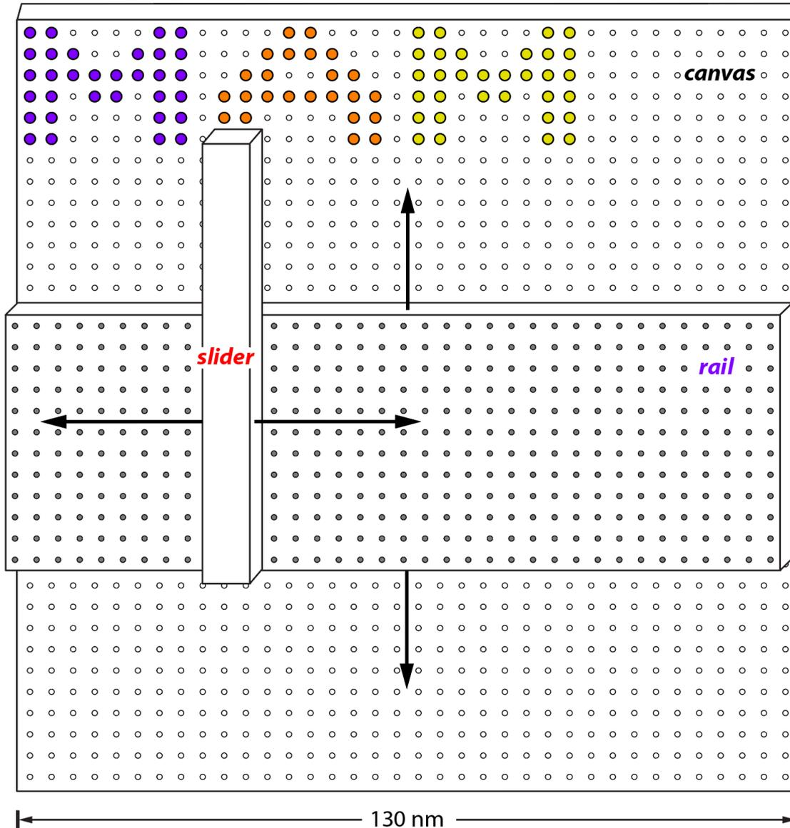
Stepper motors move **3.5 nm** per transition in response to externally triggered pulses of short DNA strands.
