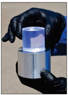
Figure 2-3. A new melt-casting fabrication process for organic glass scintillators pioneered by Sandia National Laboratories, requiring less than 24 hours and no mechanical polishing after casting, results in new crystals, such as the 2-inch diameter specimen here, capable of providing best-in-class gamma and neutron radiation discrimination capabilities.
