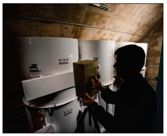
Figure 2-5. SNL designed new radiation detection equipment for New START Treaty monitoring. This new equipment detects neutron levels to confirm that objects are nonnuclear, consistent with the provisions of the treaty. (Photo by Randy Montoya)
