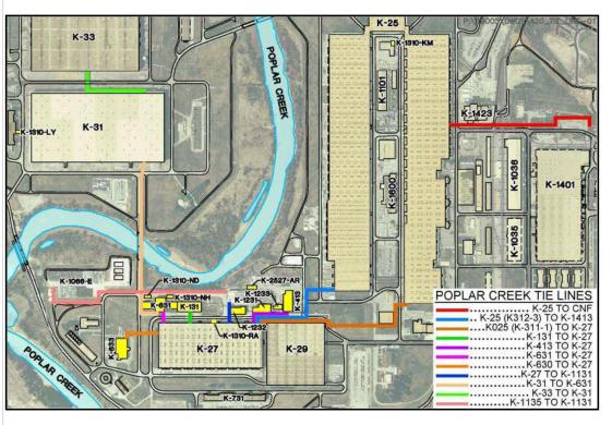
Poplar Creek facilities were located north and west of Building K-27 and primarily supported operations in Buildings K-27 and K-29. The demolition project also included removal of approximately 12,000 linear feet of process gas and utility tie lines associated with the Gaseous Diffusion Plant Facilities.
