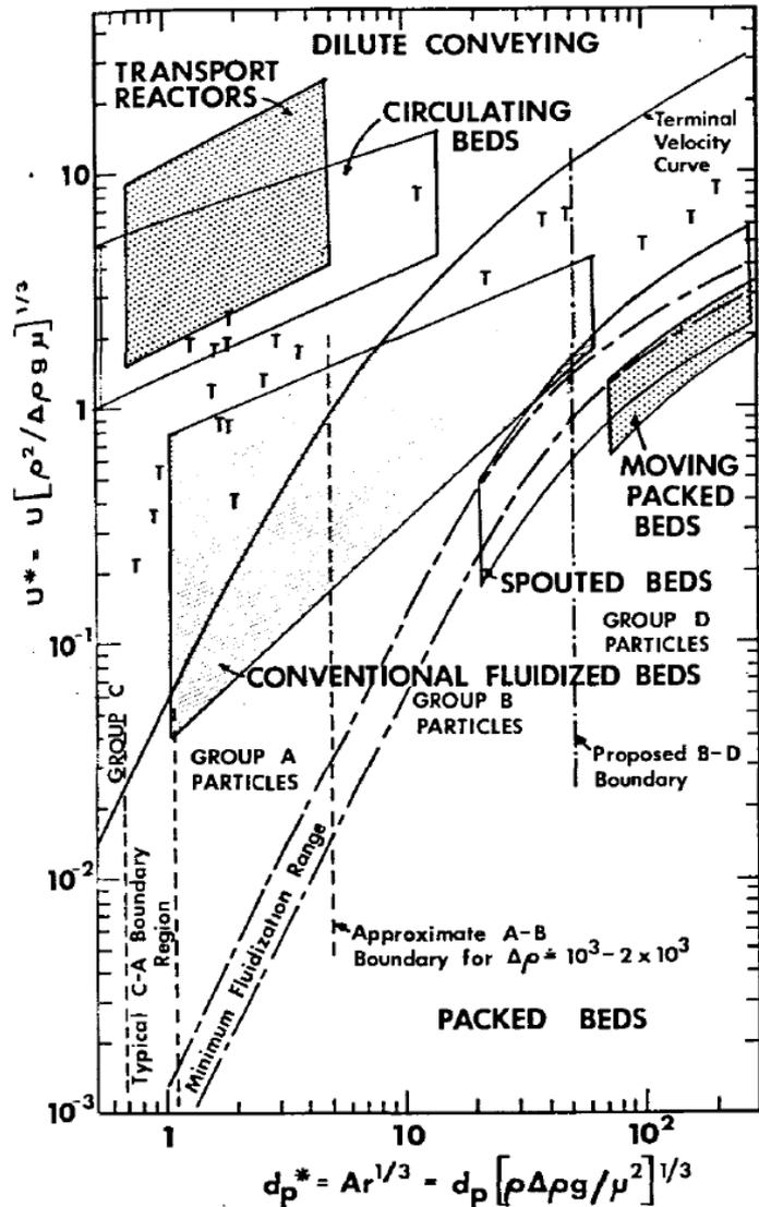
Grace developed a fluidization map based on non-dimensional flow velocity vs. non-dimensional particle size.
