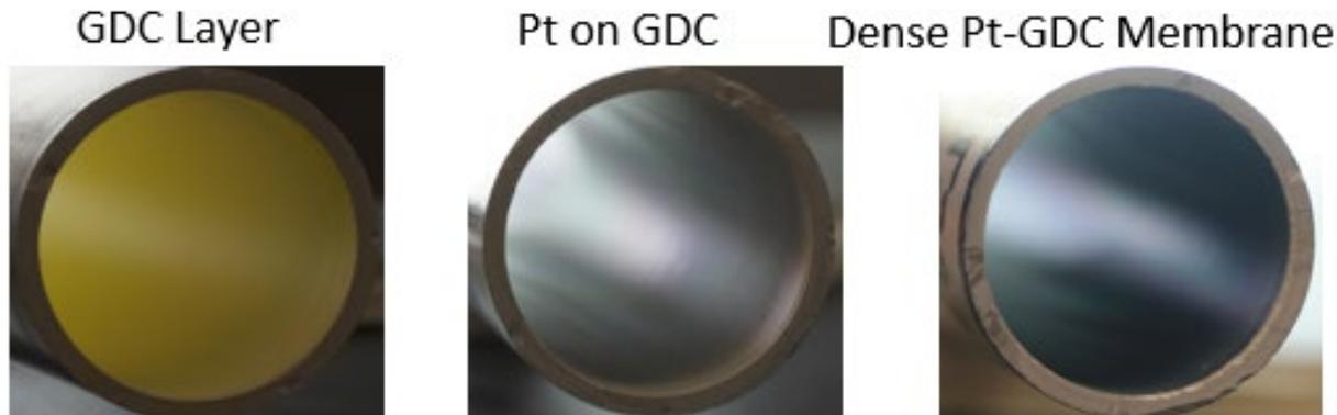
Tubular Nano-Layered Oxygen Separation Membranes
