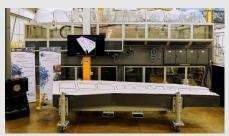
In 2016, ORNL's BAAM printed the world's largest solid 3D-printed object: a trim-and-drill tool for Boeing.
