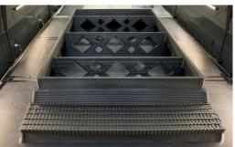
3D printed precast concrete mold (9' long x 5.5' wide) printed on the BAAM system at ORNL's Manufacturing Demonstration Facility. Photo: ORNL
