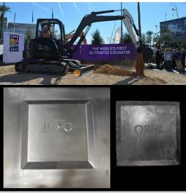
Top: The printed excavator stick – made of 927 layers printed continuously over 5 days – illustrated a 1.1mm height resolution in the Wolf Platform. Bottom: The same platform used to print the excavator stick demonstrated fabrication of steel dies for compression molding.
