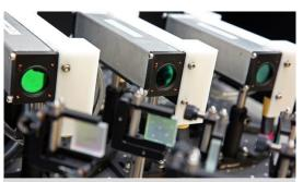
Diode-based Additive Manufacturing (DiAM) uses high-powered arrays of laser diodes and a specialized laser modulator developed for the National Ignition Facility (NIF) to flash print an entire layer of metal powder at once.
