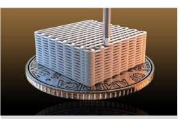
Image of graphene aerogel microlattice produced by a 3D printing technique known as direct ink writing.
