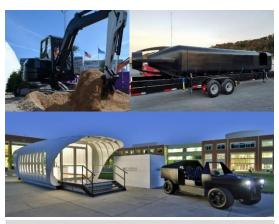
Images (clockwise from top-left): fullyfunctional AM-fabricated excavator; 3D-printed submarine; and AM-developed home and natural gas vehicle.
