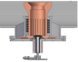
Close-up of pour tube and gas nozzle Image: Ames Laboratory
