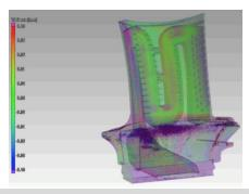
Using advanced characterization techniques and modeling to understand variance in AM builds for high temperature gas turbines.
