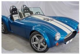
Using carbon fiber-enhanced polymers, the BAAM printer produced the frame and body of a full-scale Shelby Cobra in 2014; body panels feature a surface variation of 0.020 inches. Photo: ORNL
