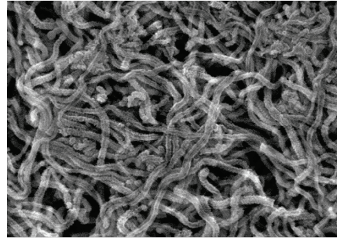
Appearance of nano-wires in battery after 10 charge-discharge cycles
