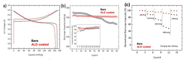
ALD nanocomposite coating improves stability and rate performance of LiCoO<sub>2</sub> cathode cells
