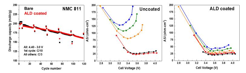
ALD nanocomposite coating reduces/maintain the impedance of NMC811 cathode cells
