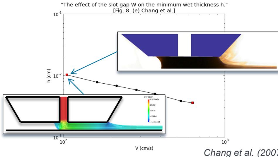
Single-layer slot-die deposition model validation: Pattern of streamlines (lower left) and published flow visualization
