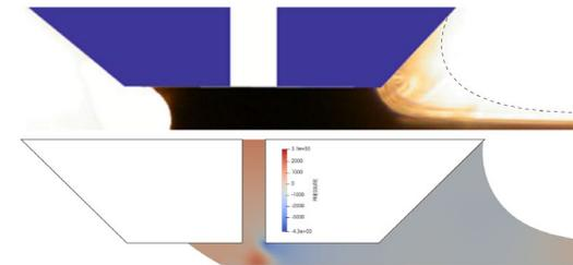
Validation of single-layer slot coating deposition (flow visualization in literature)
