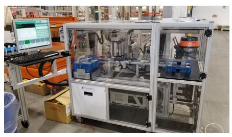
RUV-AS system in solar module production
