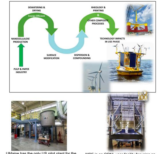
UMaine has the only US pilot plant for the production of cellulose nano-fibrils (CNFs) at 1 ton/day and patented technology for the spray drying of CNFs with ongoing research to scale this technology for mass production. MDF is an ORNL user facility focusing on cost-shared early-stage applied R&D and a leader in the areas of additive manufacturing. It has 35 systems and \$12M of industry-provided equipment.
