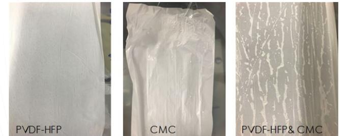
Ceramic coating on separator with various binders
