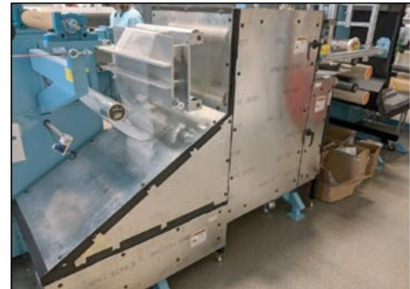
Front of the laser safety enclosure built onto the NREL diagnostic roll-to-roll system
