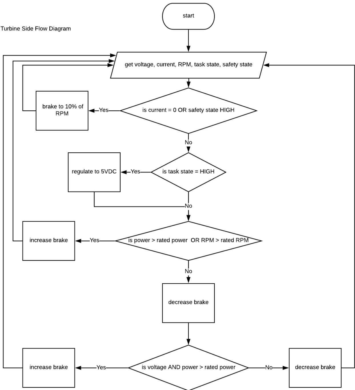
Figure 3. Flow Chart for the Turbine Side
