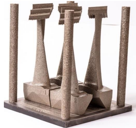
Represents IN738 turbine blades for industrial gas turbine engine using EBM technology.
