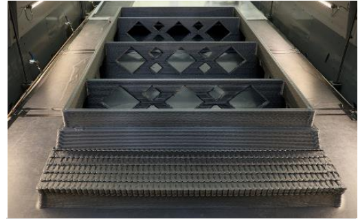
3D printed precast concrete mold (9' long x 5.5' wide) printed on the BAAM system at ORNL's Manufacturing Demonstration Facility.
