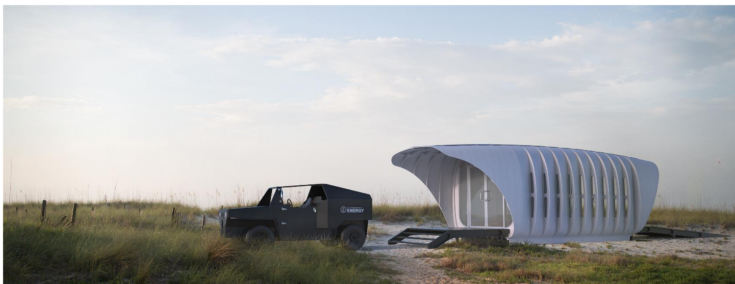
3D-printed vehicle and home developed and assembled at Oak Ridge National Laboratory's BAAM system.
