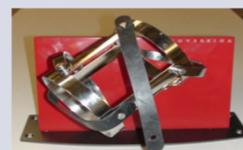
5. Can is sealed and mechanically manipulated to blend contents
