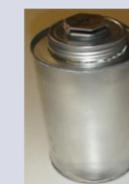
4. Pu oxide is placed in new can along with dry adulterant to dilute Pu to less than 10 weight percent
