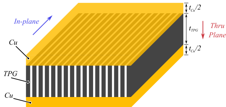
Encapsulated TPG with Cu
