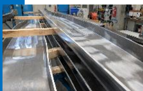
Variable Thickness Roll forming
