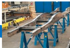
Variable Thickness Roll forming
