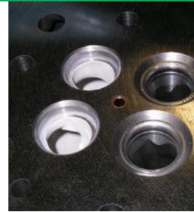
Exhaust Ports Insulation
