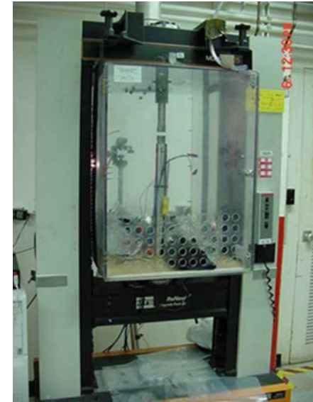
Test In Hood For Containment of Tritium Off-gassing
