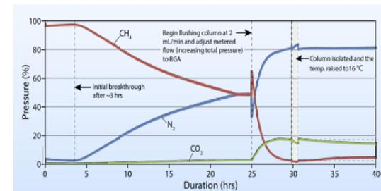
Figure 3. Partial pressure values of CO<sub>2</sub>, N<sub>2</sub>, and CH<sub>4</sub> obtained from continuous gas sampling of CH<sub>4</sub> hydrate bearing porous sand column during a titration of 90% N<sub>2</sub> and 10% CO<sub>2</sub> gas mixture.
