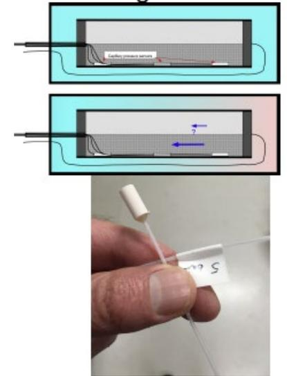
Capillary Pressure Sensor for use in geomechanical evaluation
