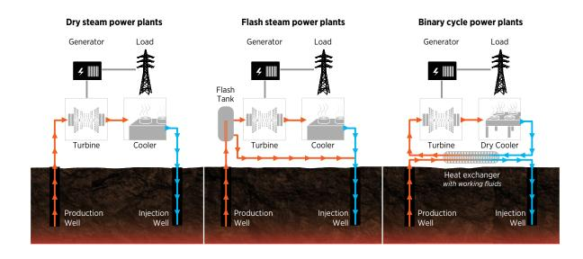
Figure 2-8. Geothermal power-plant configurations: dry steam, flash steam, and binary cycle
