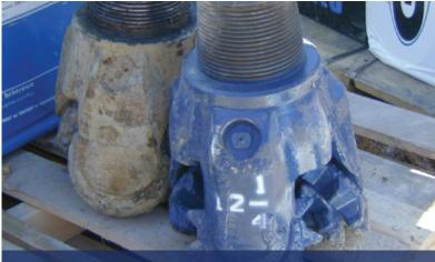
Drill bits used at the Raft River geothermal site in Idaho. Photo credit: K.T. Hanna
