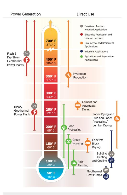
Figure 2-7. The continuum of geothermal energy technology applications and uses
