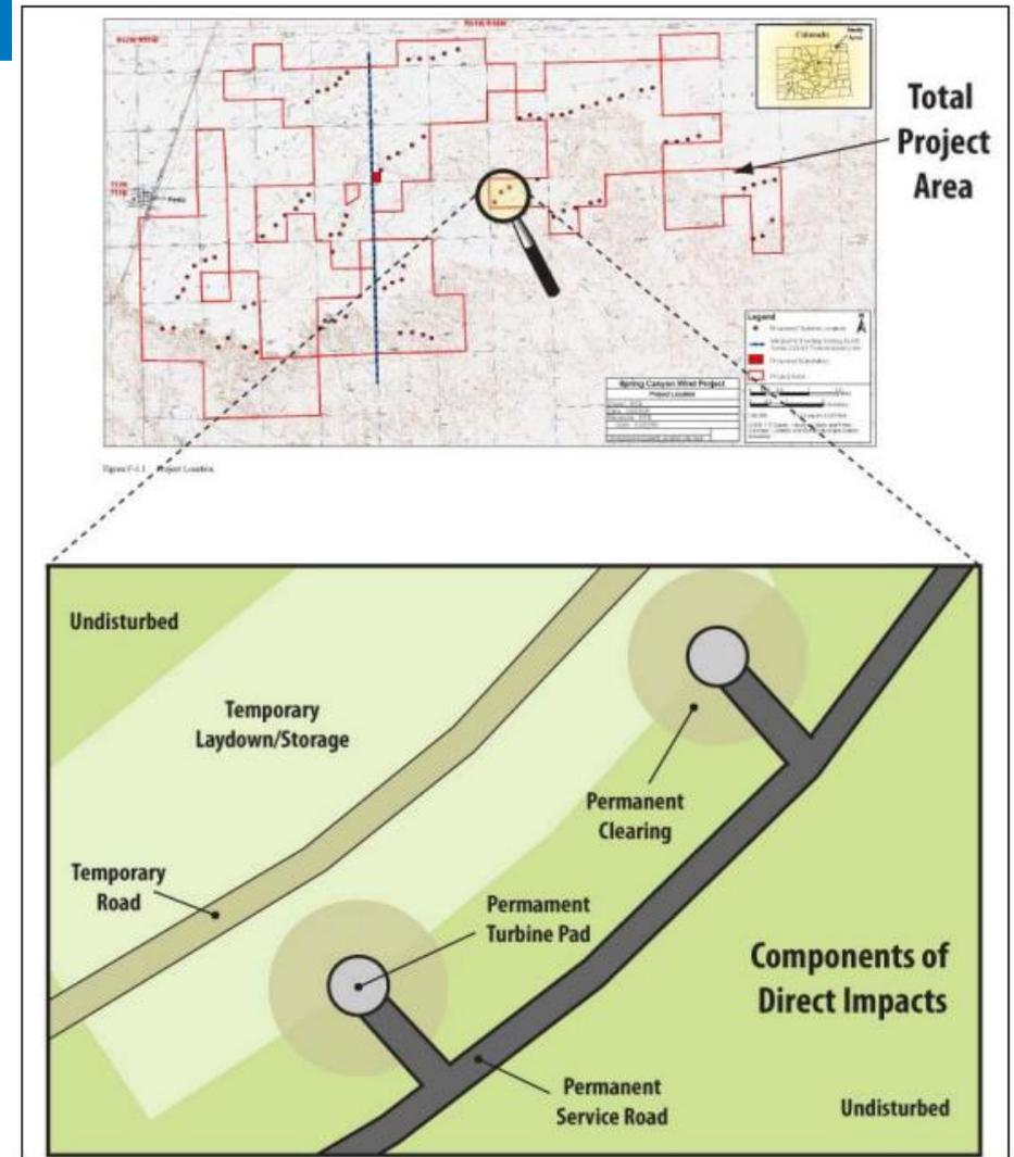
Figure 1. Illustration of the two types of wind plant land use: total area and direct impact area (including permanent and temporary)<sup>1</sup>
