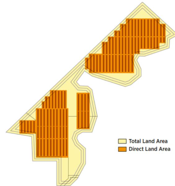
In addition to the area covered by the PV array, additional land area is required for setbacks, access roads, fencing, and a possible substation.
