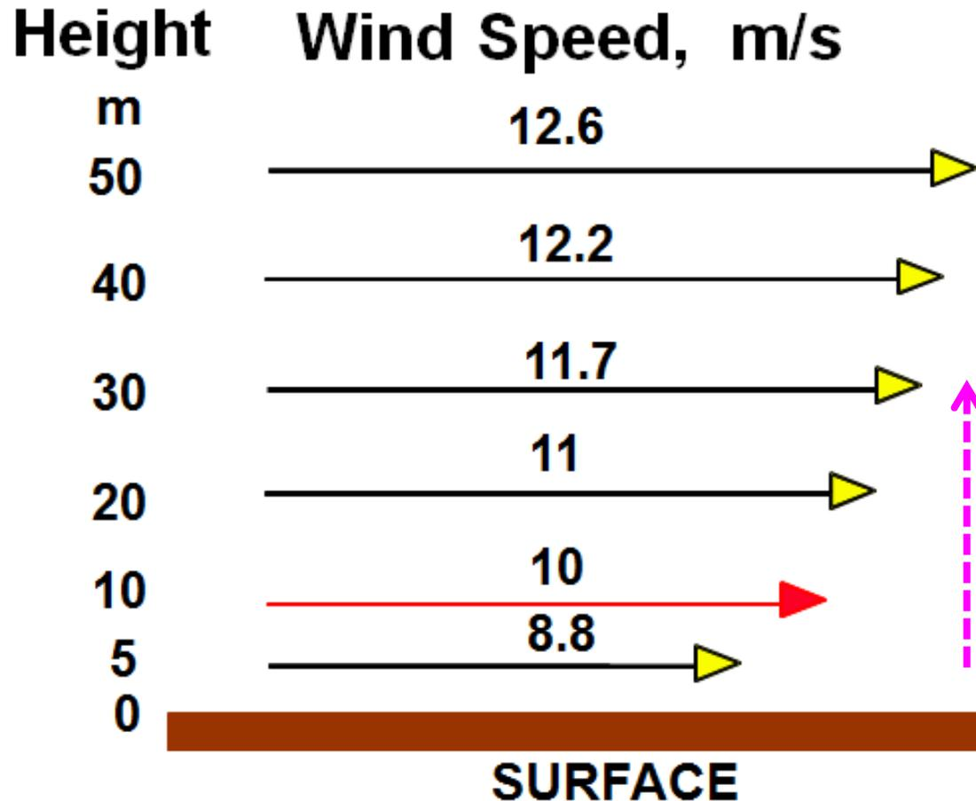
Increasing the wind speed from 8.8 to 11 m/s (25% increase), doubles the available power in the wind!
