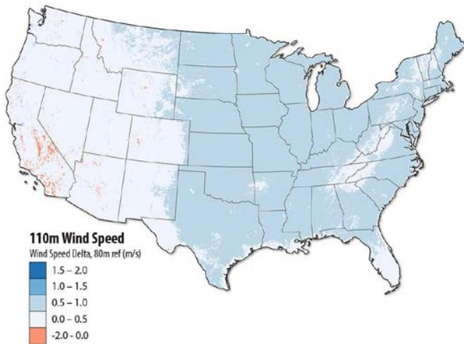
Difference in mean annual wind speed 110 m above ground level minus 80 m. Figure by NREL, based on the Wind Integration National Dataset Toolkit
