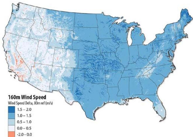
Difference in mean annual wind speed 160 m above ground level minus 80 m. Figure by NREL, based on the Wind Integration National Dataset Toolkit
