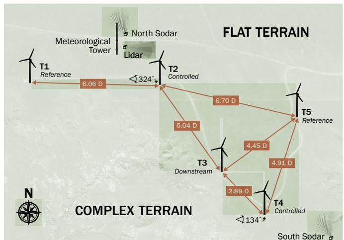
NREL measured the impact of steering individual turbine wakes away from downstream turbines at NextEra Energy Resource's Peetz Table Wind Energy Center. These field trials demonstrated increased overall energy production at the commercial scale. Figure by Paul Fleming, NREL
