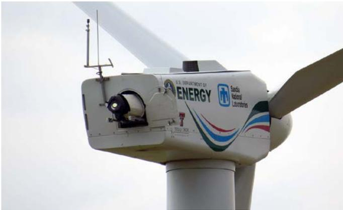
SpinnerLidar instrument installed on a SWiFT turbine. Photo by Sandia
