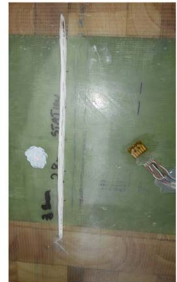
Figure 10.3. Damage introduced to the 2.8 m LP spar cap
