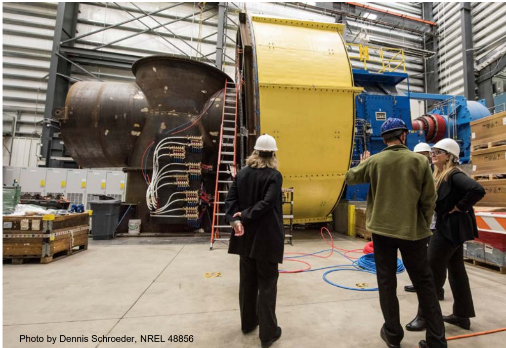
Columbia Power Technology's wave energy device generator installation in NWTC 5-MW dynamometer facility
