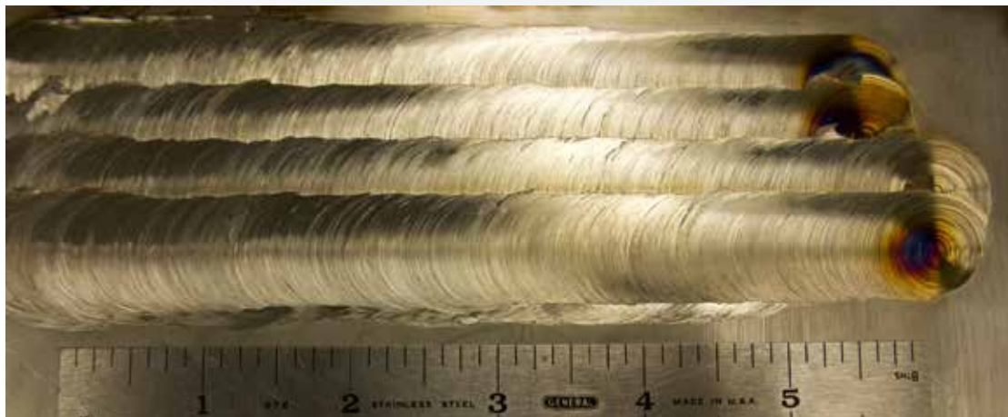
Figure 4. Process scaling up. Successful FSAM cladding with 1" diameter tool.
