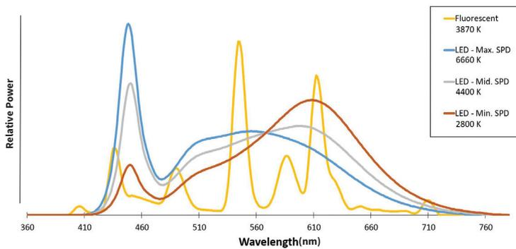
Figure 2: SPDs for three of the color control settings of the LED system and for the existing fluorescent system, measured directly underneath a luminaire installed in a classroom.
