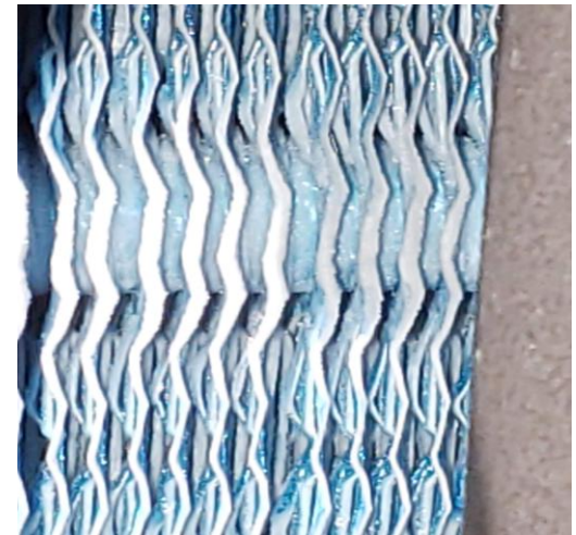
Frost growth on the evaporator of HPWH
