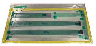
MSU Aligned Strand infusions are useful for comparing fiber properties while minimizing manufacturing effects
