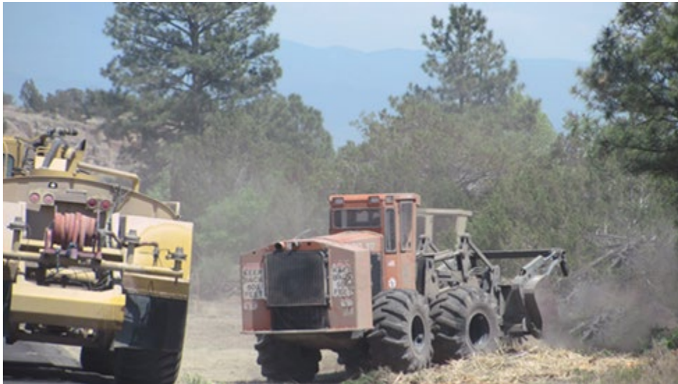
Figure 2-1 Masticators used to chip biomass in place
