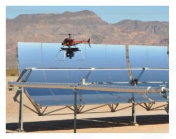
Deployment of the Aerial Distant Observer Tool to Survey Optical Performance of CSP Parabolic Trough Solar Fields
