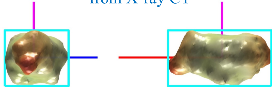
Particle reconstruction from X-ray CT
