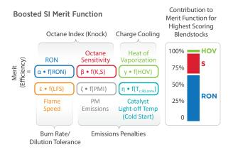
This made it possible to identify 10 blendstocks from four chemical families—alcohols, olefins, furans, and ketones—with the greatest potential to increase boosted SI efficiency. Collectively the Co-Optima research and analysis has led to a much-improved understanding of the trade-offs of fuel costs, engine technologies, and fuel economy.
