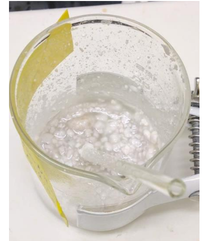
Nitrate/Expanded Perlite composite phase change material
