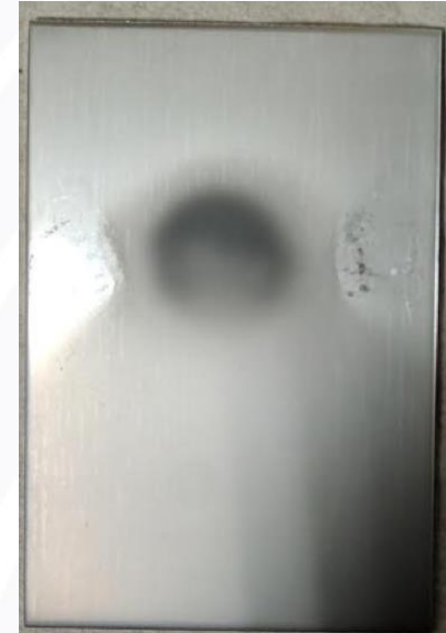
Stainless steel coupon after being impacted by 50 Kg (left), and 300 Kg (right) of HSP 40/70 in hourglass apparatus
