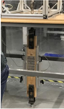
Truss joint setup
