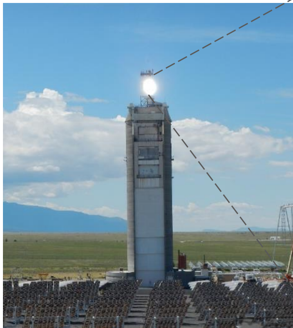
On-sun particle receiver testing at the National Solar Thermal Test Facility at Sandia National Laboratories, Albuquerque, NM
