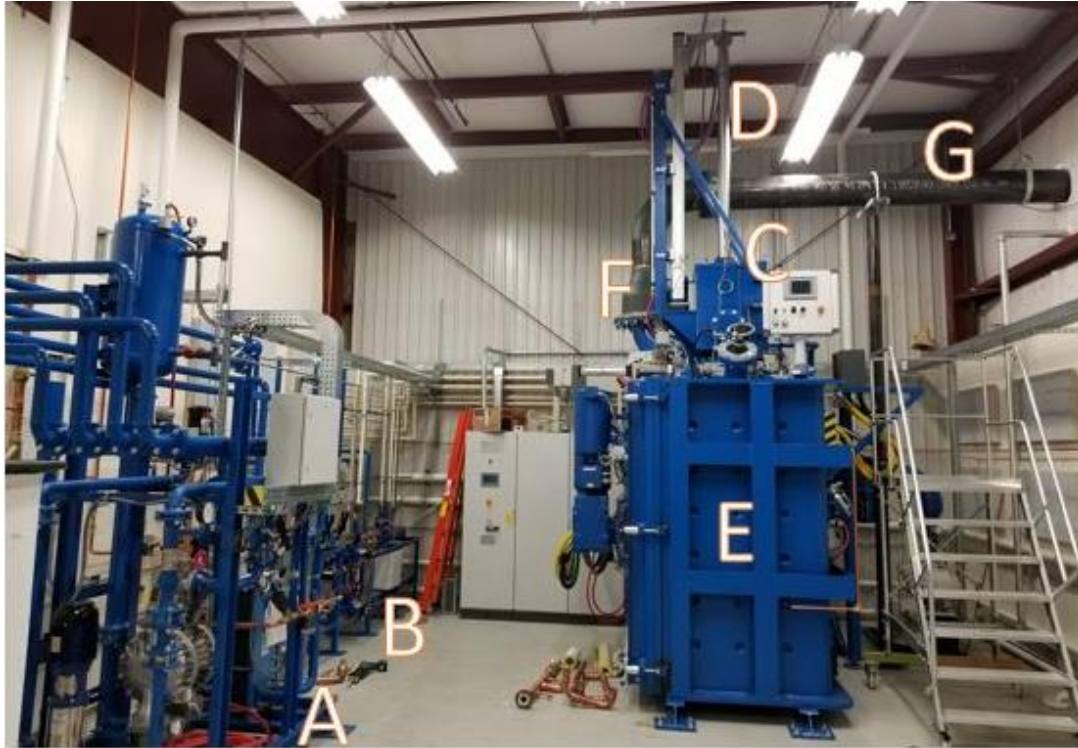
Cold-wall, Induction-heated Melt Infiltration System
