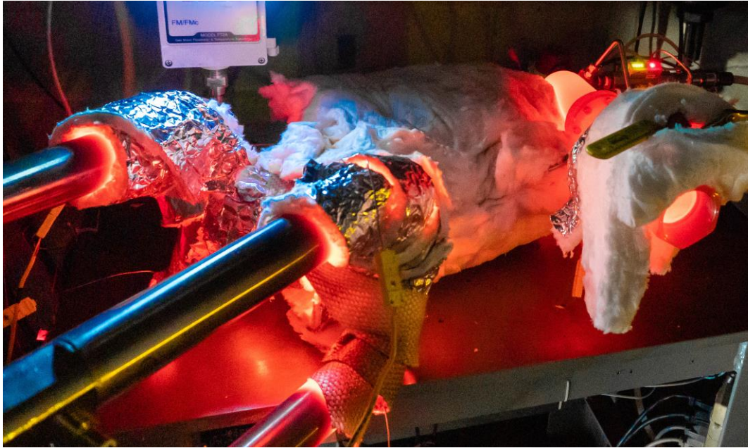
High Temperature Recycle Blower with 700°C Inlet Air
