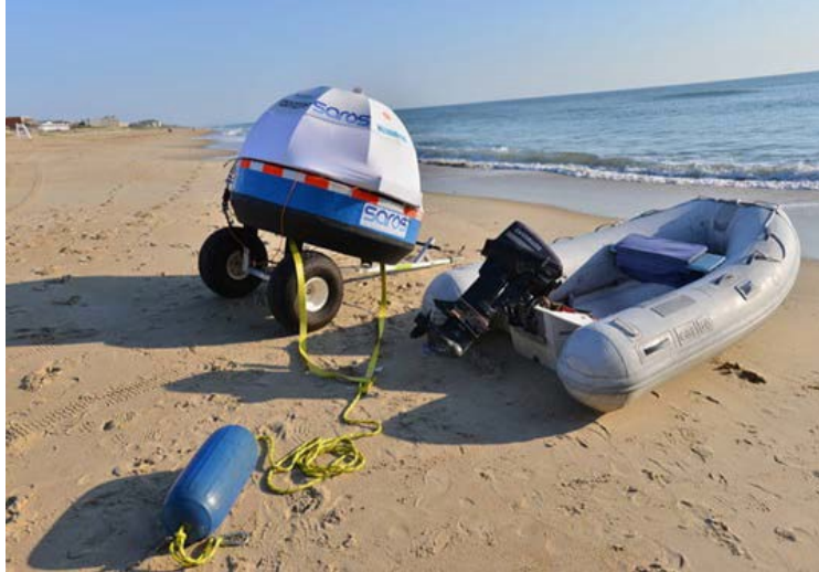
Figure 7.4. SAROS wave-powered desalination demonstration unit
