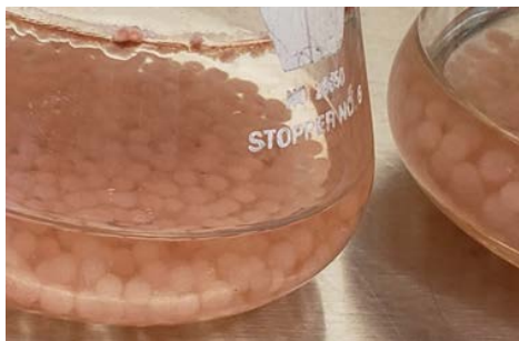
Above, right: Comparison of HPLC measurements to Raman-based PLS predictions of glucose and xylose concentrations in a culture of A. pseudoterreus fungi growing in DMR hydrolysate medium in a 30-liter bioreactor (far left image). Above, center: Photograph of an A. pseudoterreus grown in defined media shows “pellet” morphology typical of this species when grown in submerged culture.
