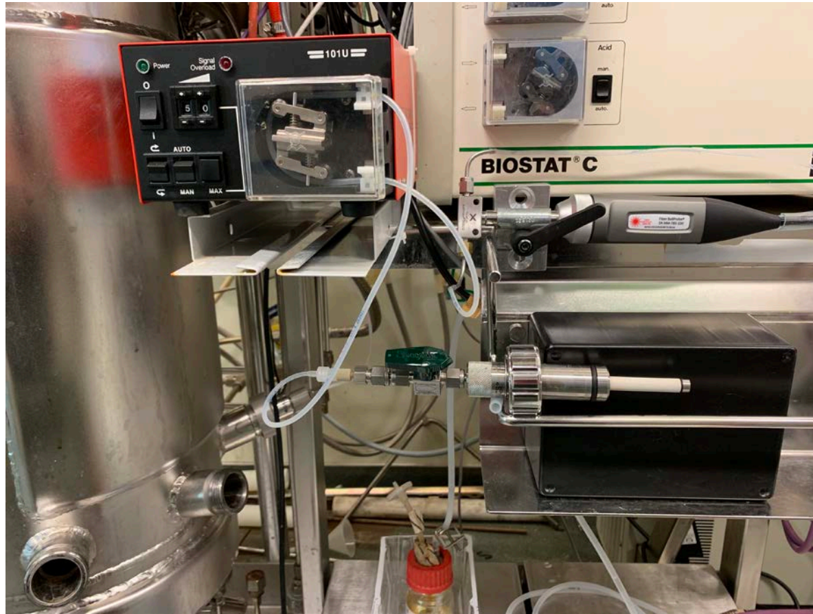
MarqMetrix BallProbe Raman flow cell detector and Flownamics FISP probe for drawing 0.2 \mu\text{m} -filtered bioreactor broth samples.
