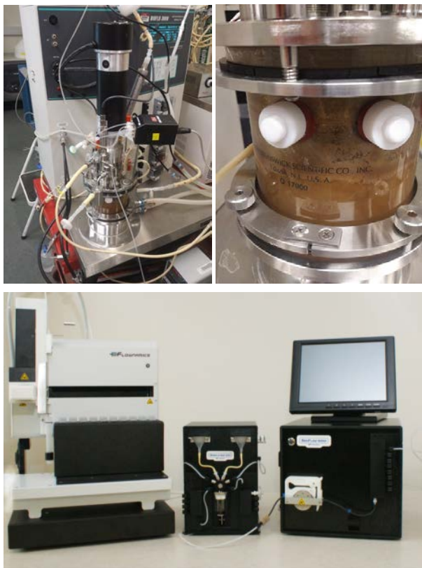
Above, left: 1.75 L bioreactor culture of A. pseudoterreus used for Raman PLS model development. Below, left: FlowNamics autosampling system used for drawing 0.2 mm-filtered samples every 30 minutes over 36 hours for Raman and HPLC data acquisition. Above, right: Plot of glucose concentrations measured by HPLC vs. Raman training and test dataset predictions via PLS.
