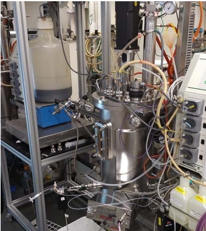
Fed-batch bioreactor setup with hydrolysate reservoir on a stir plate to keep lignin solids in suspension.
