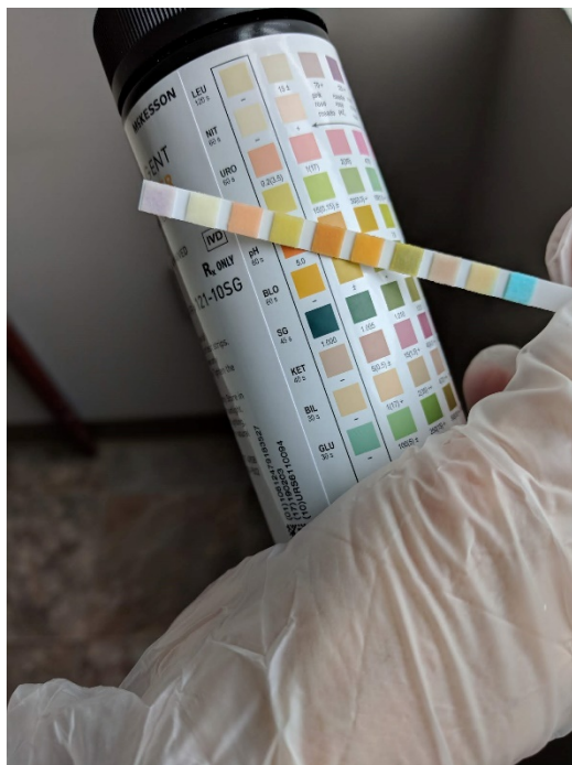
Figure 9. Example of a urinalysis test that relies on metamerism. Depending on the light source, the diagnosis can change.
