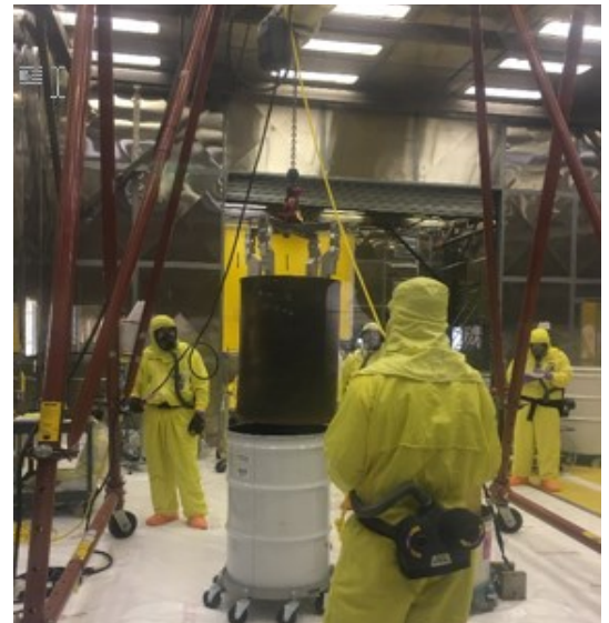
Drum liners containing UNS waste were repackaged prior to treatment.
