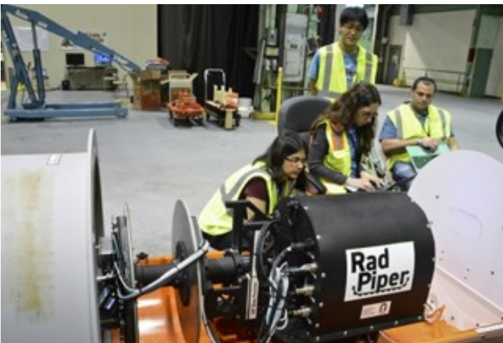
RadPiper, a pipe-crawling robot specialized for autonomous measurement of U-235 deposits, deployed in July.
