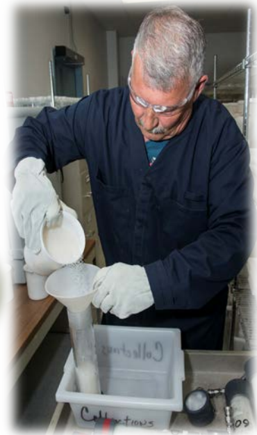
Above: Technician Prepares Rain Ion Exchange Columns
