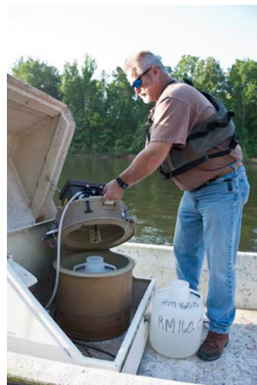
Field Technician Collects Composite River Surface Water at River Mile 160
