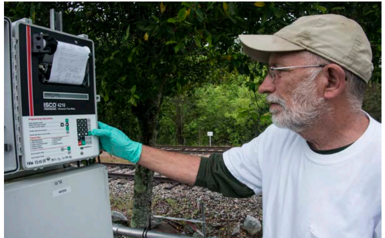
A Field Technician Verifies Flow Rate at an Industrial Wastewater Outfall
