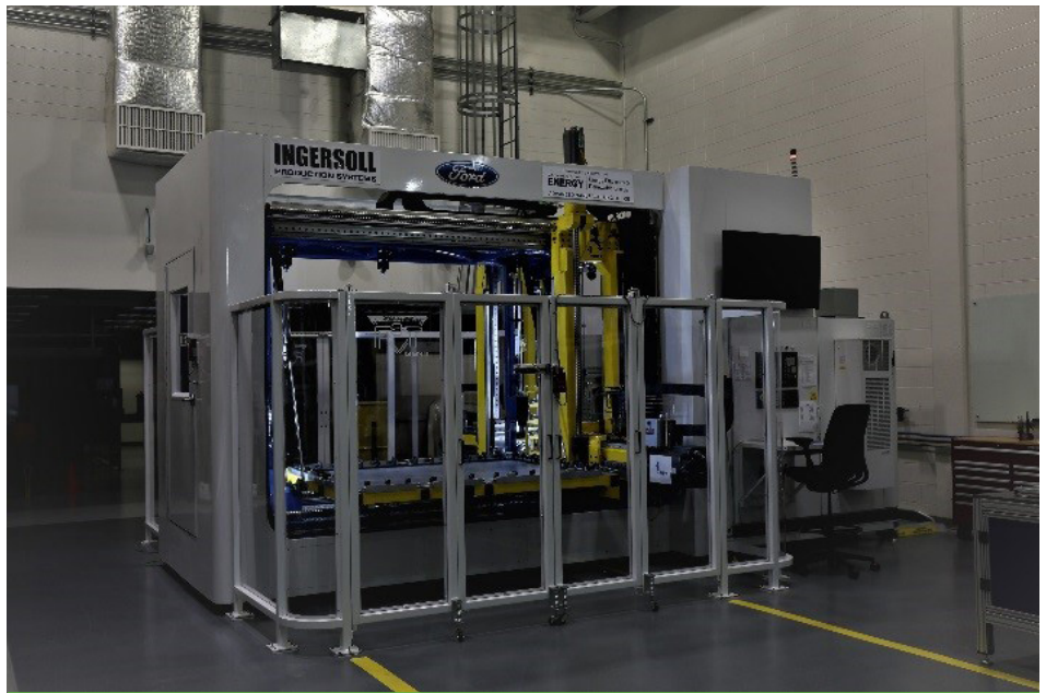
Rapid Freeform Sheet Metal Forming Technology (RAFFT) machine in Rockford, Illinois. Photo courtesy Ingersoll Rand.
