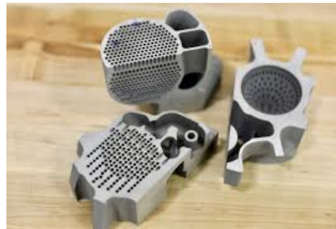
AM Heat exchanger (GE)
