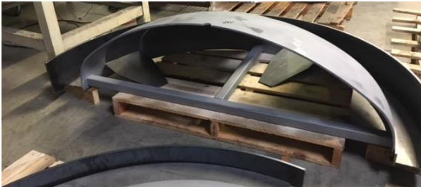
3/8-inch (9.5mm) thick lower head construction;
