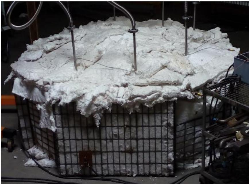
Hot Degassing of Powder Filled Upper Head
