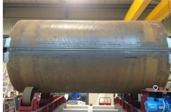
**65mm (thick) x 3m length x 1.8m diameter**
