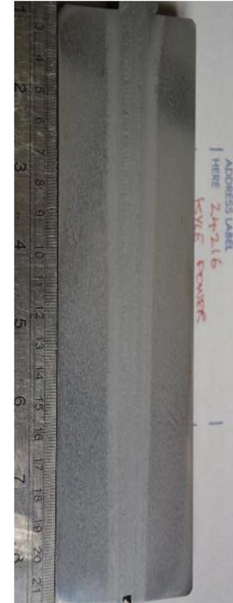
200mm Electron Beam Weld
